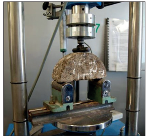
Fig. 3. The SCB test scheme
