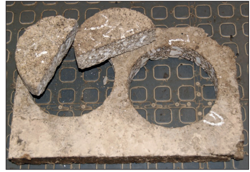
Fig. 1. Semi-cylindrical samples drilled from a compacted slab
