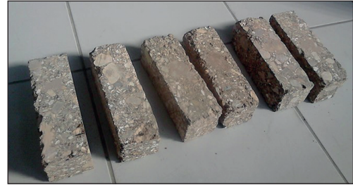
Fig. 4. Samples cut from a compacted slab
