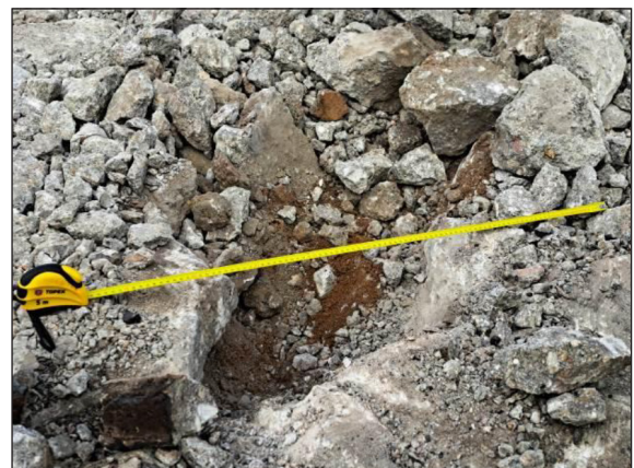
Fig. 5. Verification of the depth of stress relief in the cement concrete layer [9]
