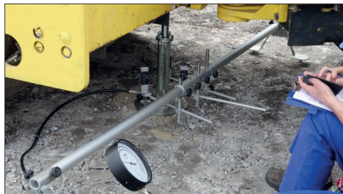
Fig. 8. Bearing capacity test with the VSS apparatus on one of the test sections [9]
