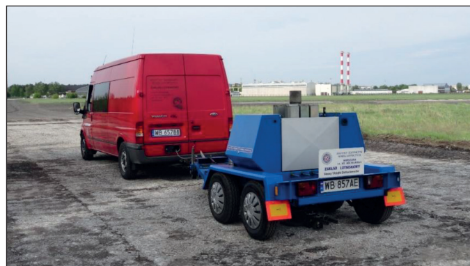
Fig. 9. Bearing capacity test with the HWD device on one of the test sections [9]
