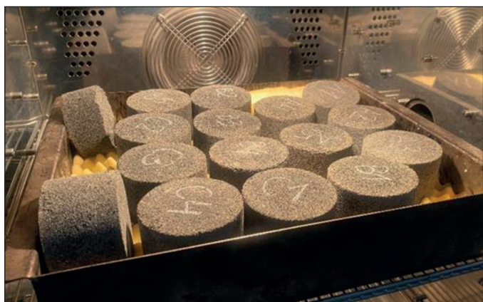
Fig. 1. Conditioning of cylindrical CSR mortar specimens
