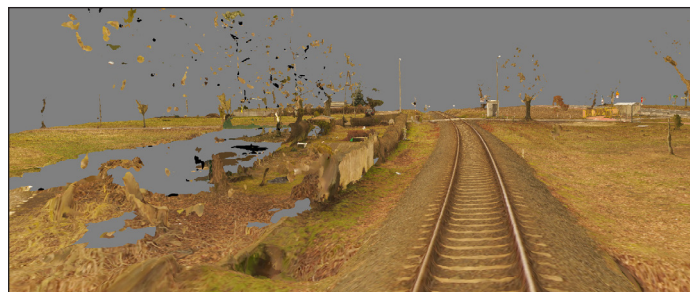
Fig. 8. View from the train driver's position (from point B, looking towards point C according to Fig. 6) generated using a 3D mesh model with textures
