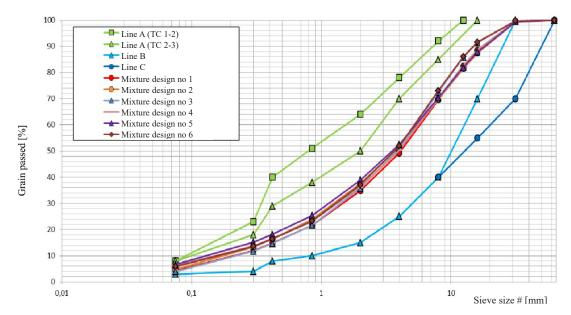
Fig.1. Graining of mineral-cement mixtures [5]
