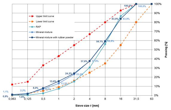
Fig. 5. MCEMRP1 coarse-grained with 0/1 mm rubber powder at the lower grain size fraction < 4 mm for medium traffic category TC $3\div4$
