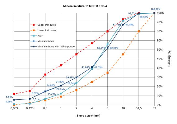
Fig. 6. MCEMRP2 medium-grained with 0/1 mm rubber powder in the middle position between the limit curves for medium traffic category TC3 $\div$ 4
