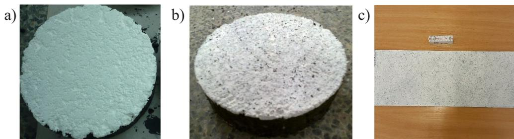
Fig. 3. Preparation of samples for DIC method testing: a) asphalt mixture sample surface painted white; b) randomly plotted black speckles; c) painted FRP sample
