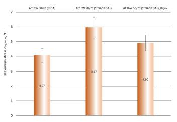
Fig. 25. TSRST maximum stress level of AC 16 W 50/70 mix after STOA ageing (control), after STOA&LTOA+ ageing and after rejuvenating treatment
