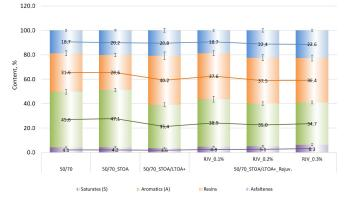
Fig. 14. Fractional compositions of 50/70 bitumen and of the bituminous binders extracted from the samples prepared for the IT-CY test
