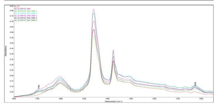
Fig. 15. Spectra of 50/70 bitumen: control, after RTFOT+PAV ageing and after rejuvenating treatment
