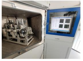
Fig. 5. 4PB-PR resistance to fatigue test of the AC 16-W-50/70 mix
