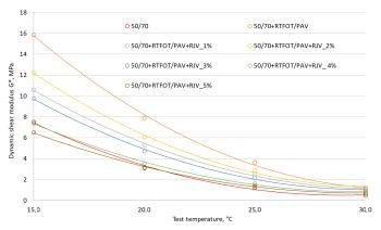
Fig. 10. Dynamic shear modulus measured in DSR for the analysed 50/70 bitumen: control, after RTFOT+PAV ageing and after rejuvenating treatment
