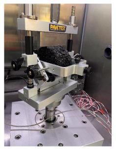
Fig. 4. Stiffness modulus determination with IT-CY test on AC 16 W 50/70 specimens
