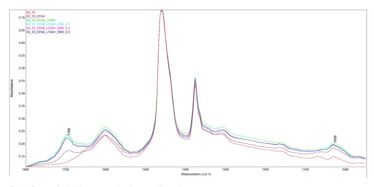
Fig. 16. Spectra of 50/70 bitumen: control and extracted from mixes
