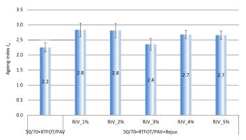
Fig. 17. 50/70 bitumen ageing index: control, after RTFOT+PAV ageing and after rejuvenating treatment
