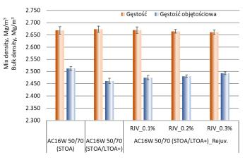
Fig. 19. Density and bulk density of AC 16 W 50/70 mix: control (after STOA), after long-term ageing (STOA&LTOA+) and after rejuvenating treatment
