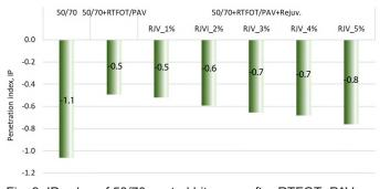
Fig. 9. IP value of 50/70 control bitumen, after RTFOT+PAV ageing, followed by rejuvenating treatment
