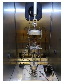
Fig. 6. TSRST test to determine low-temperature performance of AC 16 W 50/70 mix
