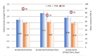
Fig. 22. Water resistance of AC 16 W 50/70 mix after STOA ageing (control), after STOA&LTOA+ ageing and after rejuvenating treatment
