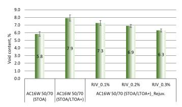
Fig. 20. Void content in AC 16 W 50/70 mix: control (after STOA), after long-term ageing (STOA&LTOA+) and after rejuvenating treatment
