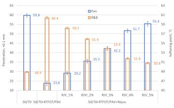
Fig. 8. Penetration and softening point of 50/70 bitumen used as a control, after RTFOT+PAV ageing, followed by rejuvenating treatment with the chosen rejuvenator
