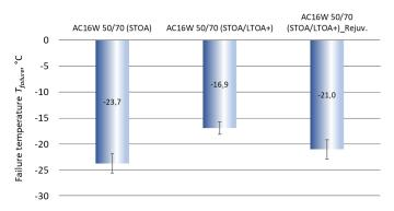
Fig. 24. TSRST failure temperature of AC 16 W 50/70 mix after STOA ageing (control), after STOA&LTOA+ ageing and after rejuvenating treatment
