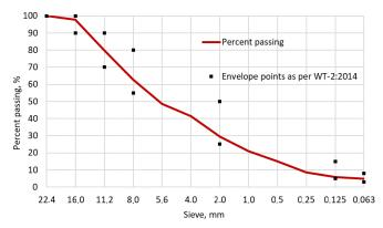
Fig. 3. Aggregate grading curve (AC 16 50/70 specified for KR3-4 medium traffic load duty class)
