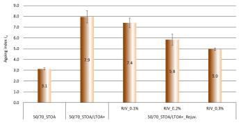
Fig. 18. 50/70 bitumen ageing index: control and extracted from RAP
