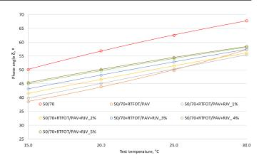
Fig. 11. Phase angle measured in DSR for the analysed 50/70 bitumen: control, after RTFOT+PAV ageing and after rejuvenating treatment
