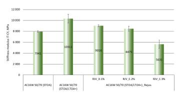
Fig. 21. Stiffness modulus of AC 16 W 50/70 mix after STOA ageing (control), after STOA&LTOA+ ageing and after rejuvenating treatment
