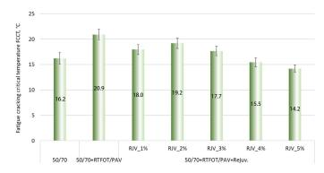
Fig. 12. Fatigue cracking critical temperature FCCT for the analysed 50/70 bitumen: control, after RTFOT+PAV ageing and after rejuvenating treatment
