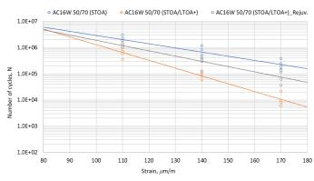
Fig. 23. Resistance to fatigue of AC 16 W 50/70 mix after STOA (control), after STOA&LTOA+ and after rejuvenating treatment
